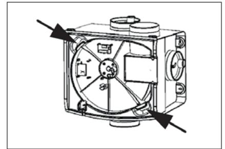
3. Remove the motor plate using the two handles (see arrows).
