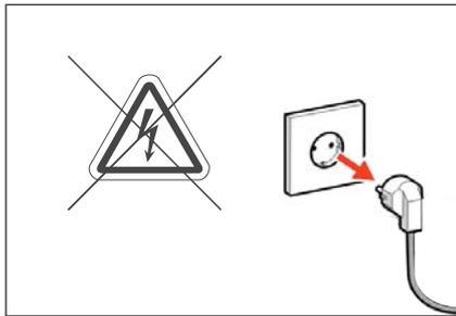
1. When maintenance is carried out the ClimaRad MaxiBox should not be connected to the power supply. Remove the plug from the socket.
