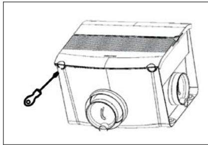
2. Remove the front cover using a flat screwdriver. Behind this cover are the electric wiring, motor and circuit board located.
