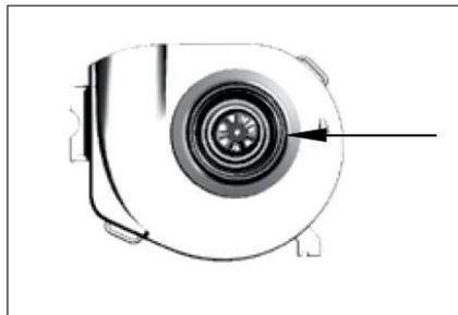
4. Inspect and clean the motor. Make sure all dirt is removed from the impeller.
