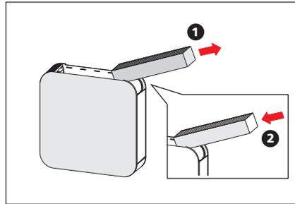
2. Remove the old filter and slide the new filter into the device. Replace the cover.
