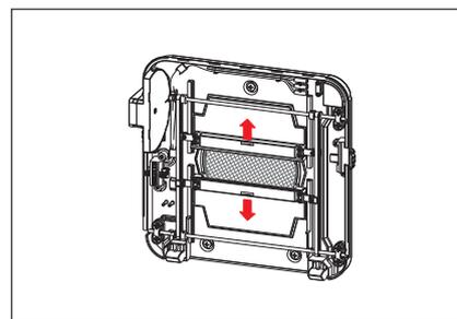
3. If necessary, open the flaps manually.
