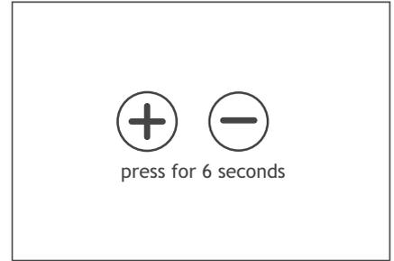
3. Reset the filter hour counter after replacement by pressing the + and - buttons on the control panel simultaneously for 6 seconds. The message "filter vervuild" should disappear.
