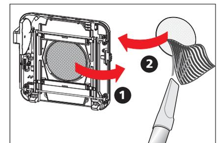
4. Remove the insect screen manually and clean it with a dry, lint-free cloth or vacuum cleaner.
