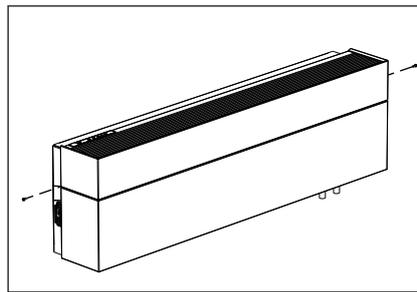
2. Unscrew the locking screws from the housing. The lower housing now moves forward.
