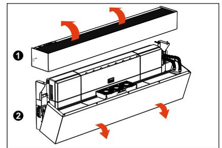
3. Loosen the screws and remove the upper housing from the unit (1). Tilt the lower housing forwards (n.b.: this is held in place with magnets.) Position it in the brackets provided for this purpose (2).
