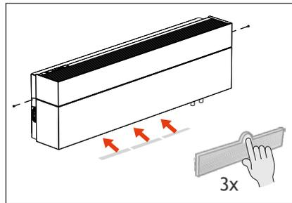
2. The output filters (3 pieces) are located at the bottom of the device, in the middle. These can be removed by placing a finger behind the notch.
