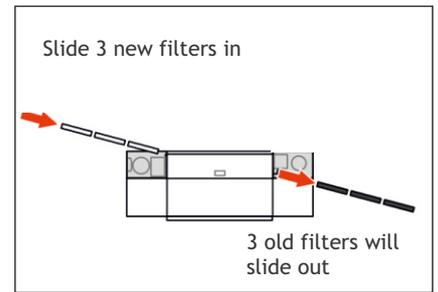
6. Slide three new filter elements into the device on the left side. The old filter elements are automatically ejected from the right side.
