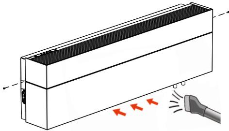
The air output filters are located at the bottom of the device. Vacuum the visible dirt off the filters. This guarantees the air flow. You do not need to remove the air output filters to do this.
