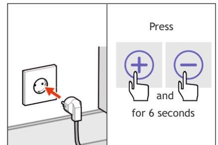
9. Put the plug back into the socket and reset the filter hour counter (Press + and - simultaneously for 6 seconds). The 'filter vervuild' message will now disappear.
