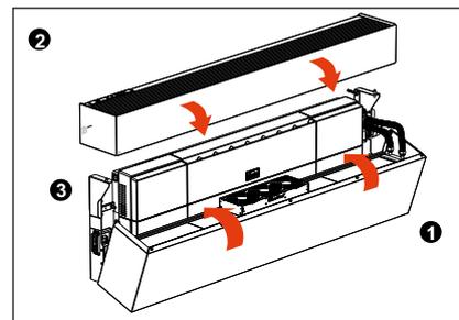
8. Reinstall the air distributor (1), tilt the lower housing back in position (2), and tighten the screws again (3).
