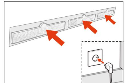
3. Push 3 new filters into the holders and then push the plug back into the socket.
