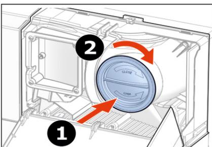
7. Push both blue filter caps back in completely in order to ensure correct operation and screw them back into position.
