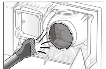
6. Remove dirt from both ducts with a vacuum cleaner or a soft cloth (do not use water).
