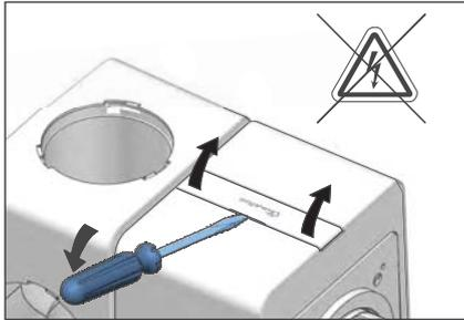
1. Disconnect the power and open the cover of the fan housing using a screwdriver.
