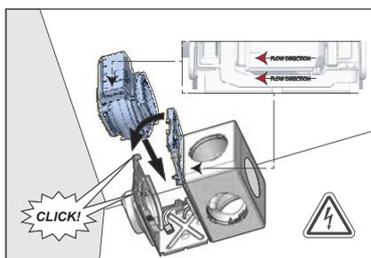
8. Push the fan back into the frame. Squeeze the sliders in the bracket and snap the bracket on both sides to close.
