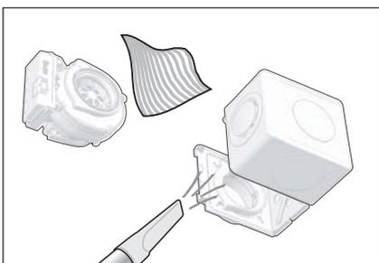
7. Remove any dirt from the channels and fan with a soft, lint-free cloth or vacuum cleaner (do not use water).
