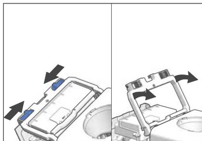
5. Push the two sliders of the bracket toward each other and tilt the bracket upwards to open.
