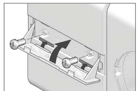
9. Insert the screws in the housing and snap the cover of the fan housing to close.
