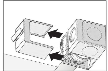
3. Remove the housing by pulling the opened cover upwards.
