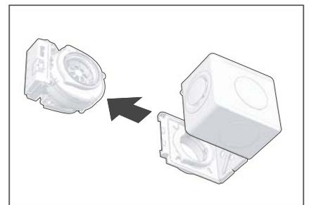
6. Remove the fan from the housing and snap the bracket back into the frame.
