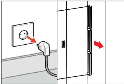
1. Pull the plug from the socket and pull the filter tray at the right side of the ClimaRad forwards.
