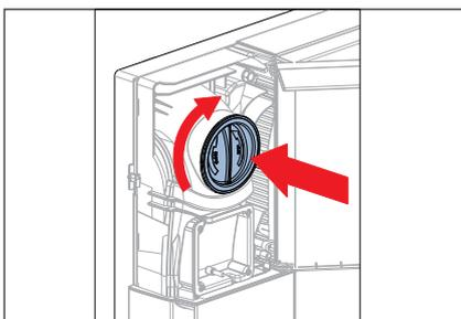
6. Push both blue filter caps fully back in for a correct operation and tighten.
