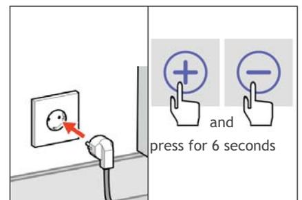
9. Push the plug back into the socket and reset the filter hour counter (by simultaneously pressing on the + and - on the display for 6 seconds). The message 'Filter vervuild' will disappear. Tighten the locking screws again.
