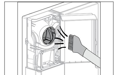
5. Remove any dirt from both channels with a vacuum cleaner or a soft cloth (do not use water).
