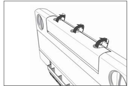
3. Open the three clips on the top and tilt the filter housing forwards.
