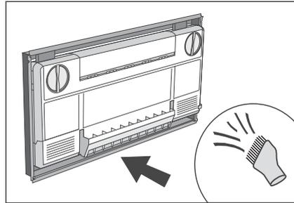
2. Use a vacuum cleaner to remove as much dirt as possible from the filter tray at the bottom.
