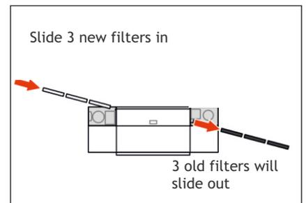
6. Slide the three new filters in the unit from the left-hand side. The old filters will automatically slide out on the right-hand side.
