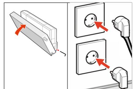
9. Unlock the radiator and tilt it back. Push the plug back into the sockets and tighten the retaining screws.
