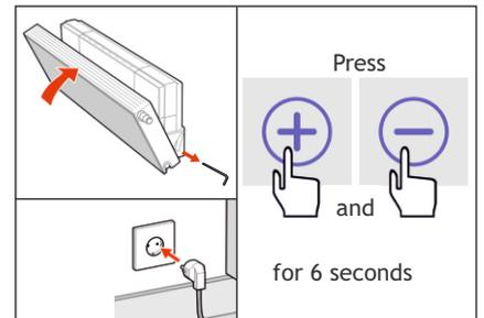
9. Unlock the radiator and tilt it back. Push the plug back into the socket and reset the filter hour counter (by simultaneously pressing on the + and - on the display for 6 seconds). The message 'Filter vervuld' will disappear. Tighten the locking screws again.
