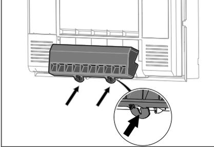
10. Press the grille at the bottom with the two clips firmly closed until you feel it snap. Please note that the filter housing must be properly closed for proper operation.
