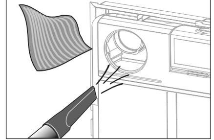
12. Remove any dirt from both channels with a vacuum cleaner or a soft cloth (do not use water).
