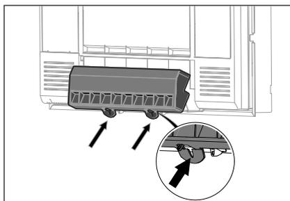
8. Replacing the air outlet filters. When the air outlet filters are dirty you need to unlock the filter housing by gently pulling the two clips towards you. Turn the filter grille as far forward as possible.
