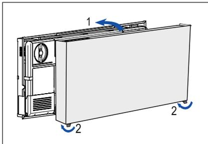
14. Put the cover back on and turn the locking hooks (at the bottom or on the side of the housing).
