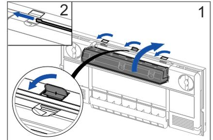
6. 1. Close the filter housing and secure with the three clips. Caution: The filters must not protrude out of the filter housing. 2. Slide the cover to the left to close.
