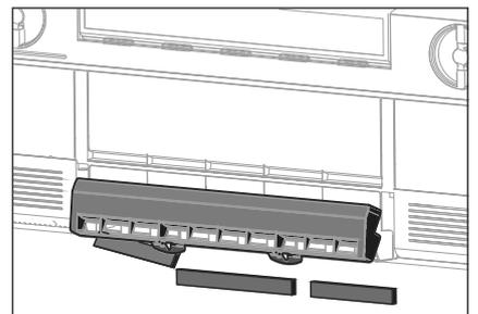
9. Push the filters from the front out of the filter housing. Place the three new filters in the sections.
