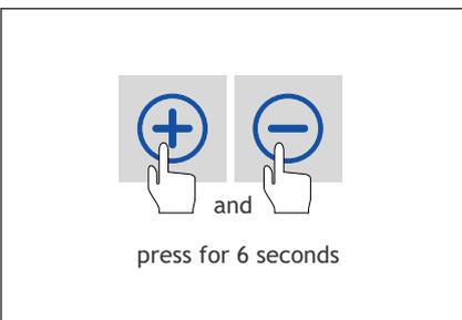
16. Reset the filter hour counter by simultaneously pressing on the + and - on the display for 6 seconds. The message 'Filter vervuild' will disappear.
