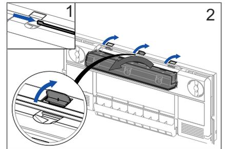
3. Replace the air supply filters. 1. Slide the cover to the right; the clips are now visible. 2. Open the three clips on the top and tilt the filter housing forwards.
