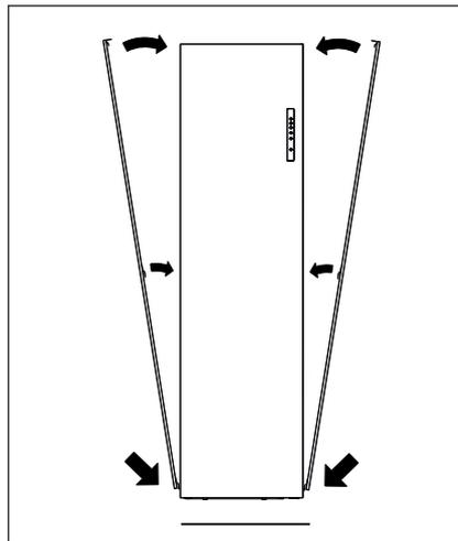
5. Place the side panel back. Then replace the two screws on the top panel.
