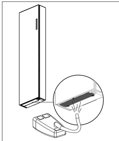
2. Clean the insect mesh at the bottom of the unit using your vacuum cleaner.
