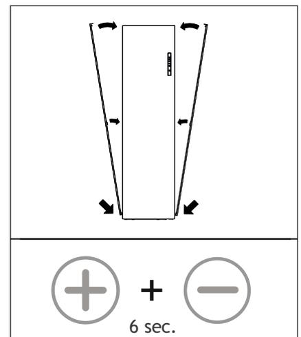
6. Place the side panel back. Then replace the two screws on the top panel. Reset the filter hour counter by holding the key combination above for 6 seconds. The "filter vervuild" notification will disappear.
