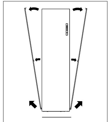
3. Remove the two screws on the top panel. Then remove one of the two side panels of the device.
