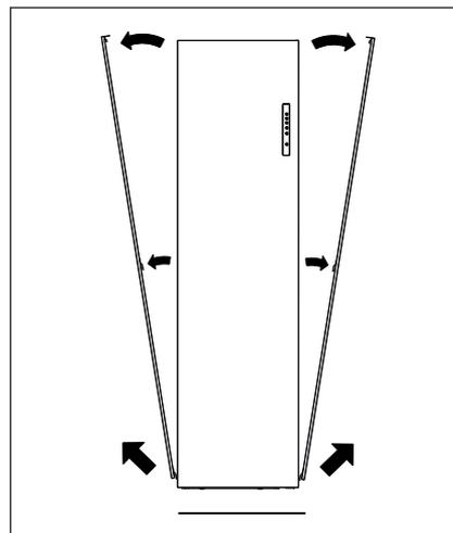
2. Remove the two screws on the top panel. Then remove one of the two side panels of the device.
