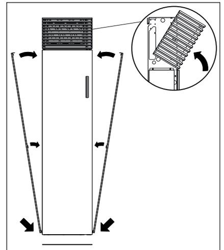
6. Place the side panel back on the device, then place the upper grille back. Press any button to leave the service mode.
