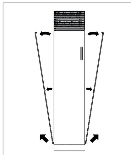
2. Remove one of the two side panels of the device.
