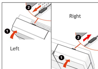
8. Close the flaps on the left and right sides of the device and slide both lock sliders back.
