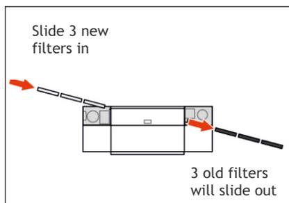
5. On the left side, slide three new filter parts into the device. On the right side, the old filter parts come out automatically.
