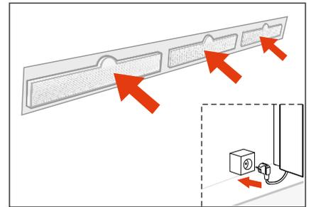
3. Push 3 new exhaust filters into the holders and then plug the plug back in.
