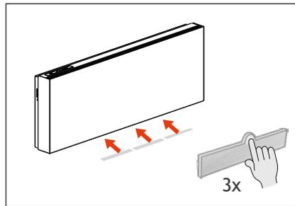
2. The 3 exhaust filters are located at the bottom of the device, in the middle. These can be removed by placing a finger behind the notch.
