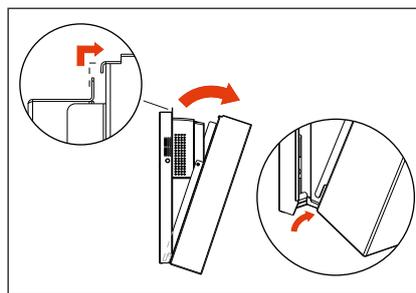
2. Remove the casing by lifting it slightly, then tilting it forward and lifting it out of the wall frame. Pay attention to the cabling of the control panel.
