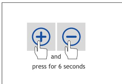
15. Reset the filter hour counter by simultaneously pressing on the + and - on the display for 6 seconds. The message 'Filter vervuild' will disappear.
