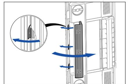
3. Air supply filters. Open the three clips at the left side and tilt the filter housing forwards.
