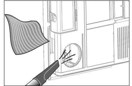
11. Remove any dirt from both channels with a vacuum cleaner or a soft cloth (do not use water).
