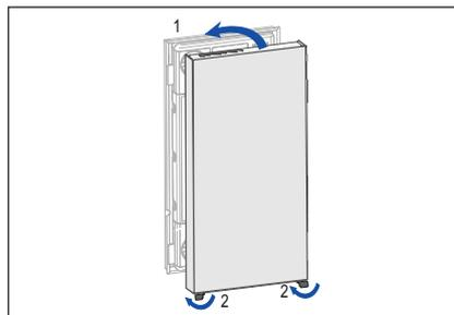
13. Put the cover back on and turn the locking hooks (at the bottom or on the side of the housing).
