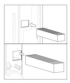
4. Remove both polluted filters and place the new inlet filter (below) and output filter (above).
