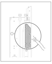
5. Clean the insect mesh on both sides of the convector using your vacuum cleaner.
