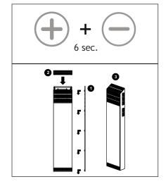
6. Reset the filter hours counter by pressing the above key combination for6 seconds. The "filter dirty" message disappears.Press any key to exit service mode.
