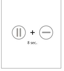
2. Set your device to service mode by holding the key combination above for 8 seconds. All LEDs will light up. Wait 1 minute for the valves to close.
