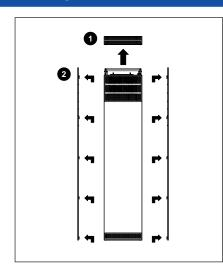
1.First remove the top grid of the appliance (1). Then the right and left side panels (2). The internal control panel is attached on the right side.
