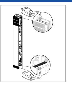
3. Clean the insect mesh at the top and bottom of the unit using your vacuum cleaner.
