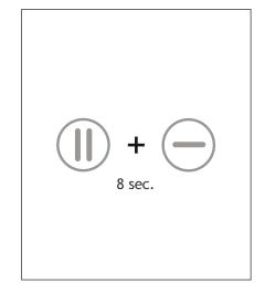
1. Set your device to service mode by holding the key combination above for 8 seconds. All LEDs will light up. Wait 1 minute for the valves to close.
