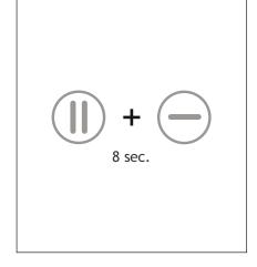
1. Set your device to service mode by holding the key combination above for 8 seconds. All LEDs will light up. Wait 1 minute for the valves to open.
