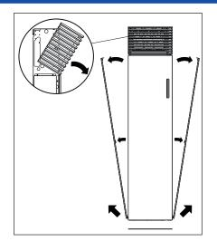
3. First remove the top grille of the device, then remove one of the side panels.
