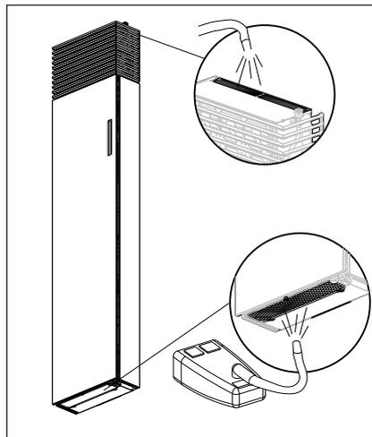
2. Clean the insect mesh at the top and bottom of the unit using your vacuum cleaner.
