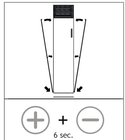
6. Place the side panel back. Reset the filter hour counter by holding the key combination above for 6 seconds. The “filter vervuild” notification will disappear.
